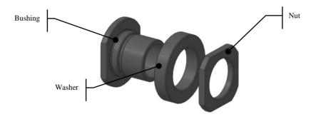
Figure 12 PROfix grinding wheel locking set
