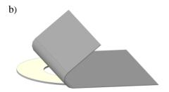
Carefully apply the abrasive paper with the abrasive face up to the adhesive surface of the metal disc. Press, smoothing the surface, squeezing out air bubbles between the disc and the abrasive paper.
