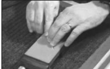
Put your hands on the blade and apply force of 10... 12 kg under axis in the area of a hole and draw the blade to yourself in order to remove burrs.
