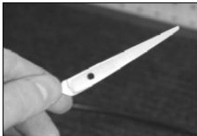
Remove moisture from limescale and wet it again. Put the blade on the limescale at 45° again and shuttle until cutting edge support line appears.
