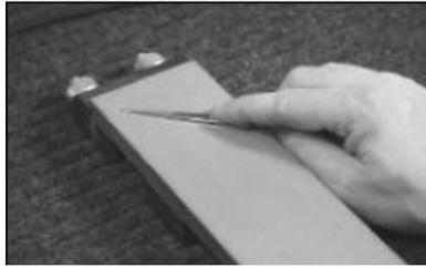
Put blade onto limescale at 45° in such a way that cutting edge is directed away from you.
