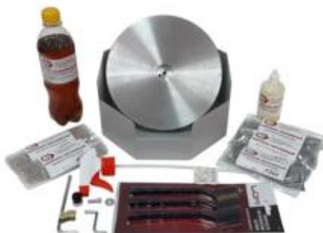
Figure 5 Set for sharpening of knife packages
