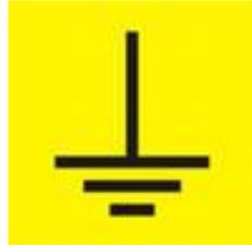
It is recommended to connect the machine to mains socket equipped with grounding wire.
